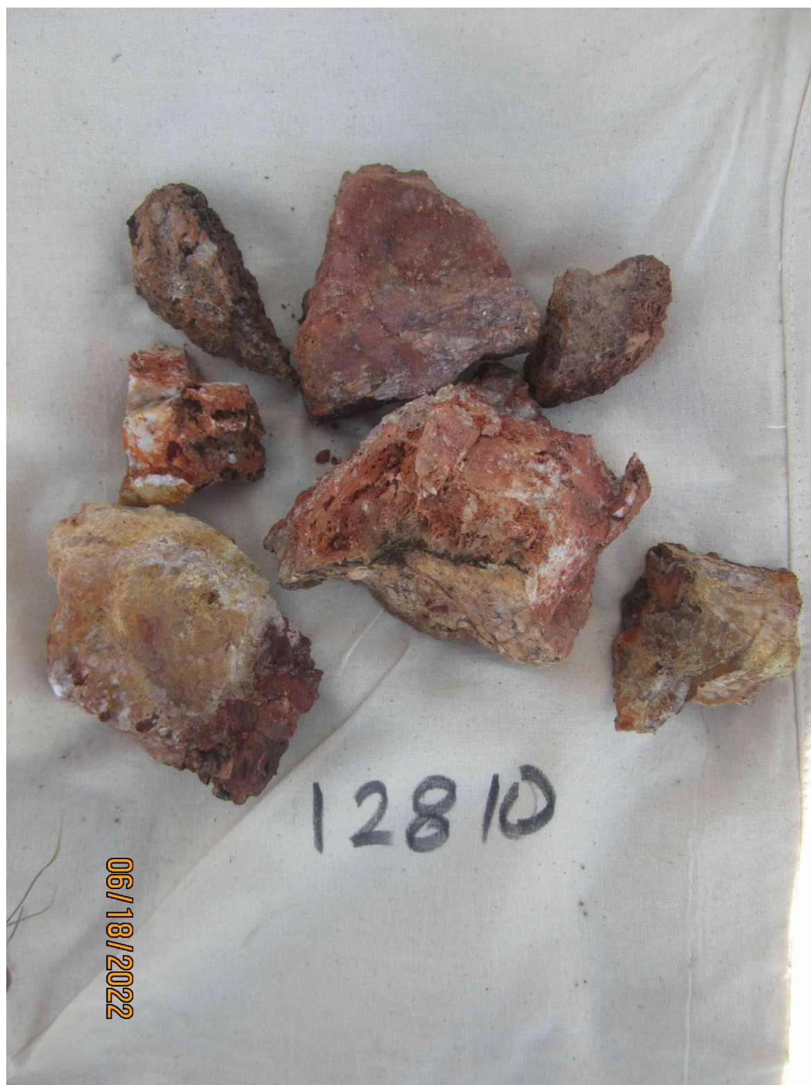
PLATE 2: Photo of composite rock chip sample from the Southeastern Silicified Ridge prospect. Sample is composed of brecciated gneiss and phyllite cemented and replaced by silica. Vughs often lined by limonite after sulphides (sample # 12810 - 31.6 g/t gold).
