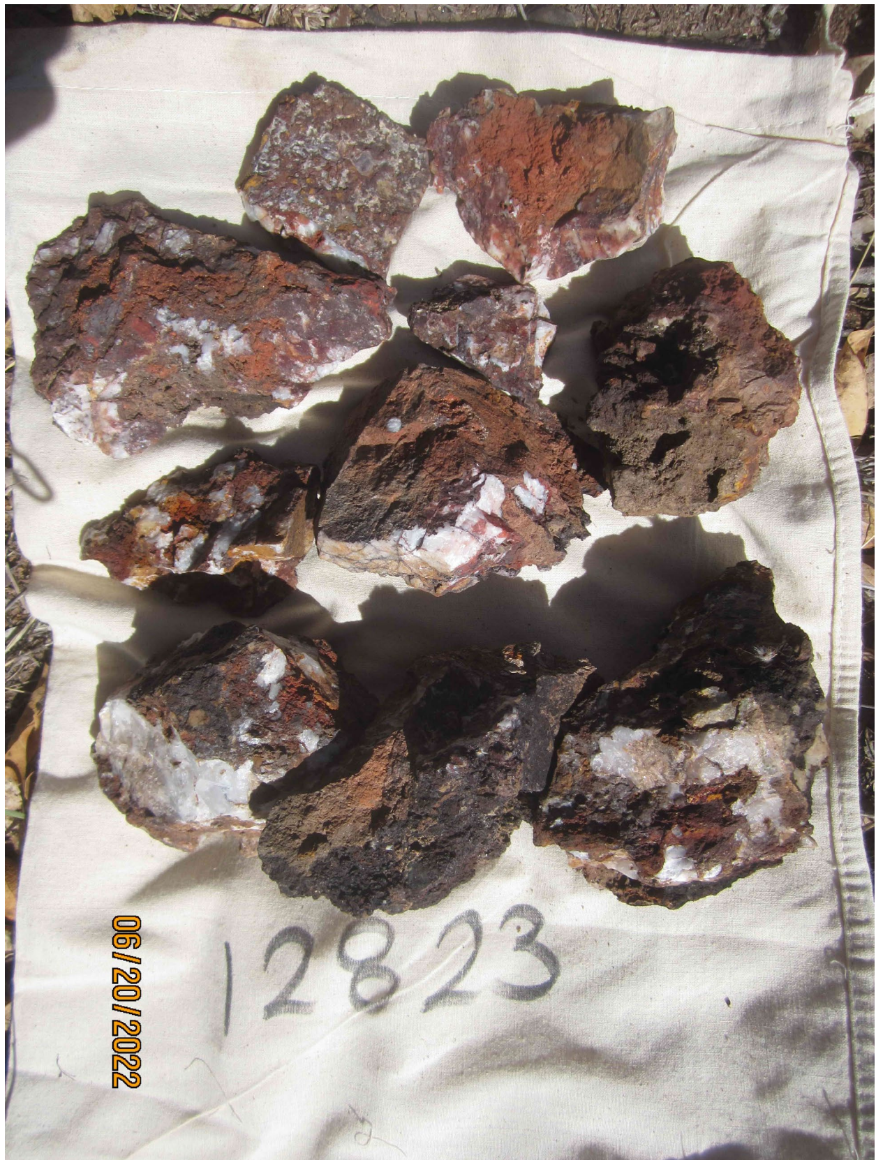
PLATE 4: Photo of composite rock chip sample from the Goldsmiths North prospect. Brecciated and silicified gneissic rock with vughs lined by limonite after sulphides and carbonate? Sample # 12823 – 18.25 g/t gold).
