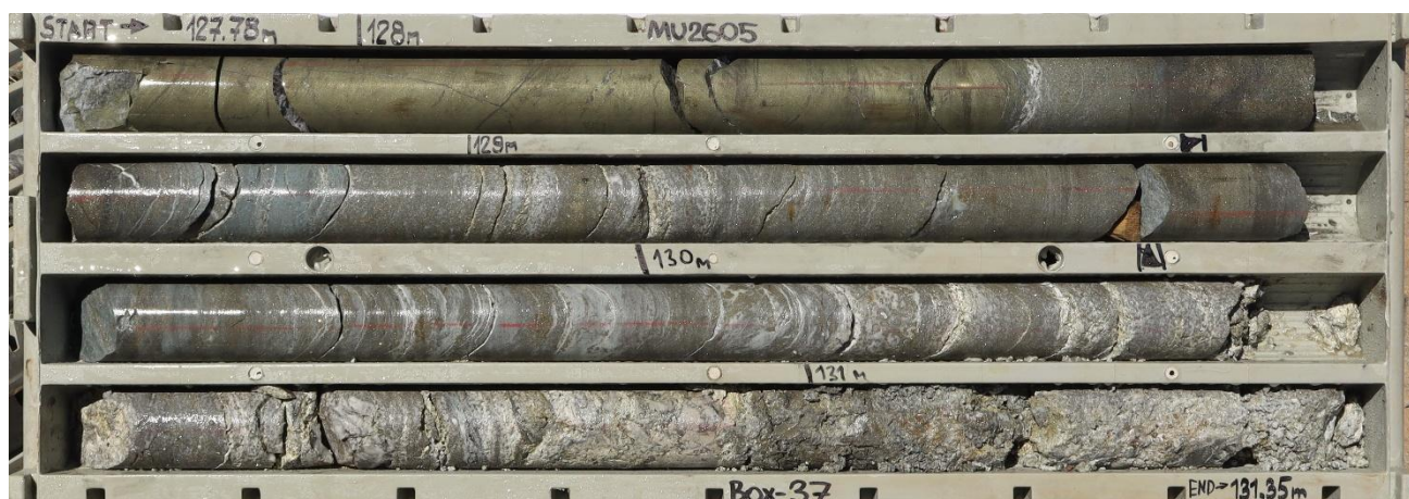
Photo 3. Massive to semi-massive sulphide zone within broader strong disseminated sulphide mineralisation, drillhole MU2605, box 37 (127.78 to 131.35 metres). Visual estimates of mineral abundance are provided in Table 2.
