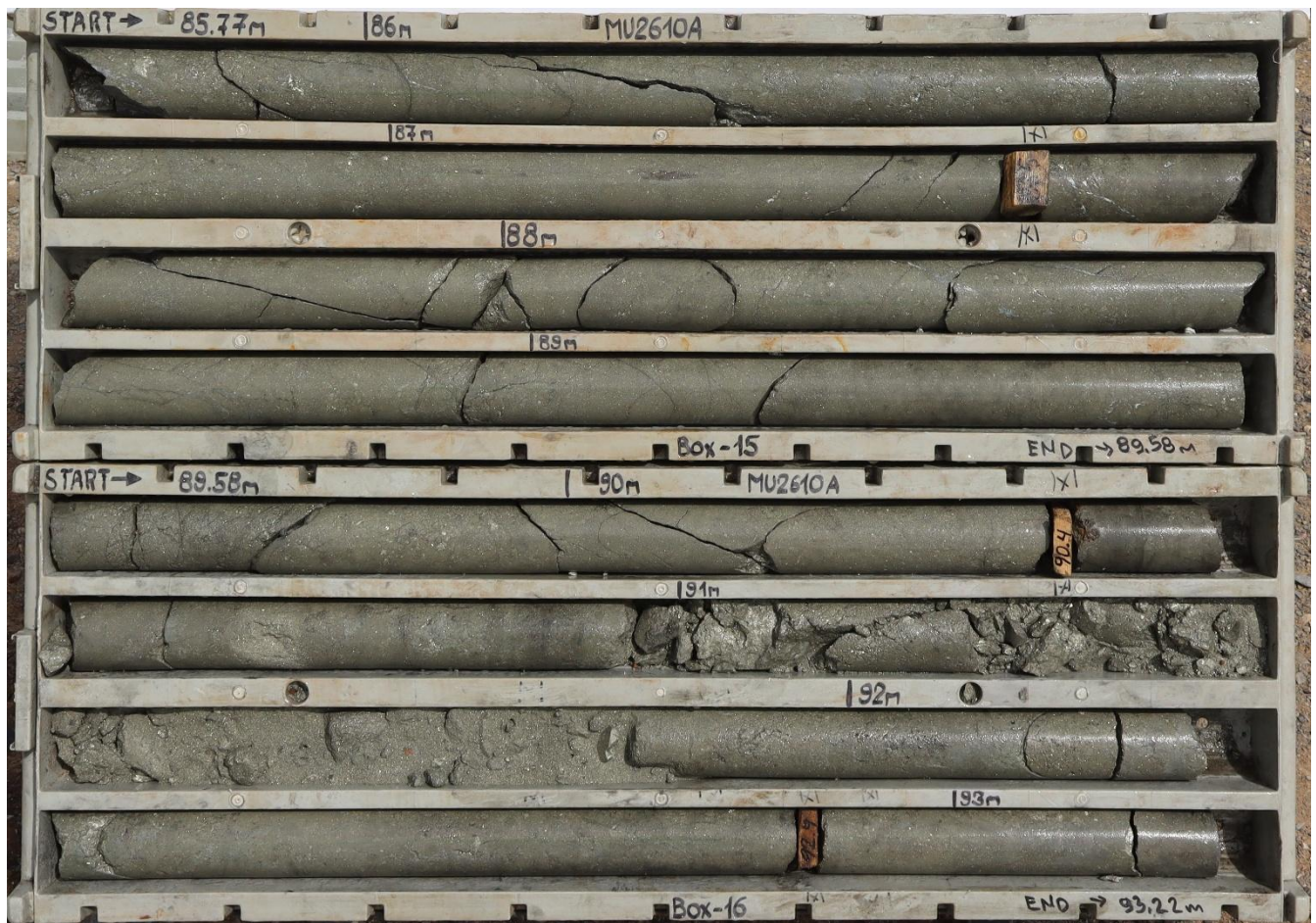
Photo 1. Massive sulphide mineralisation, drillhole MU2610A, boxes 15-16 (85.77 to 93.22 m). Visual estimates of mineral abundance are provided in Table 1.
