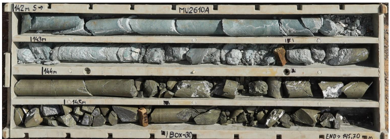
Photo 2. Chalcopyrite-rich massive sulphide mineralisation (from 143.85 m), drillhole MU2610A, box 30 (142.0 to 145.7 m). Visual estimates of mineral abundance are provided in Table 1.
