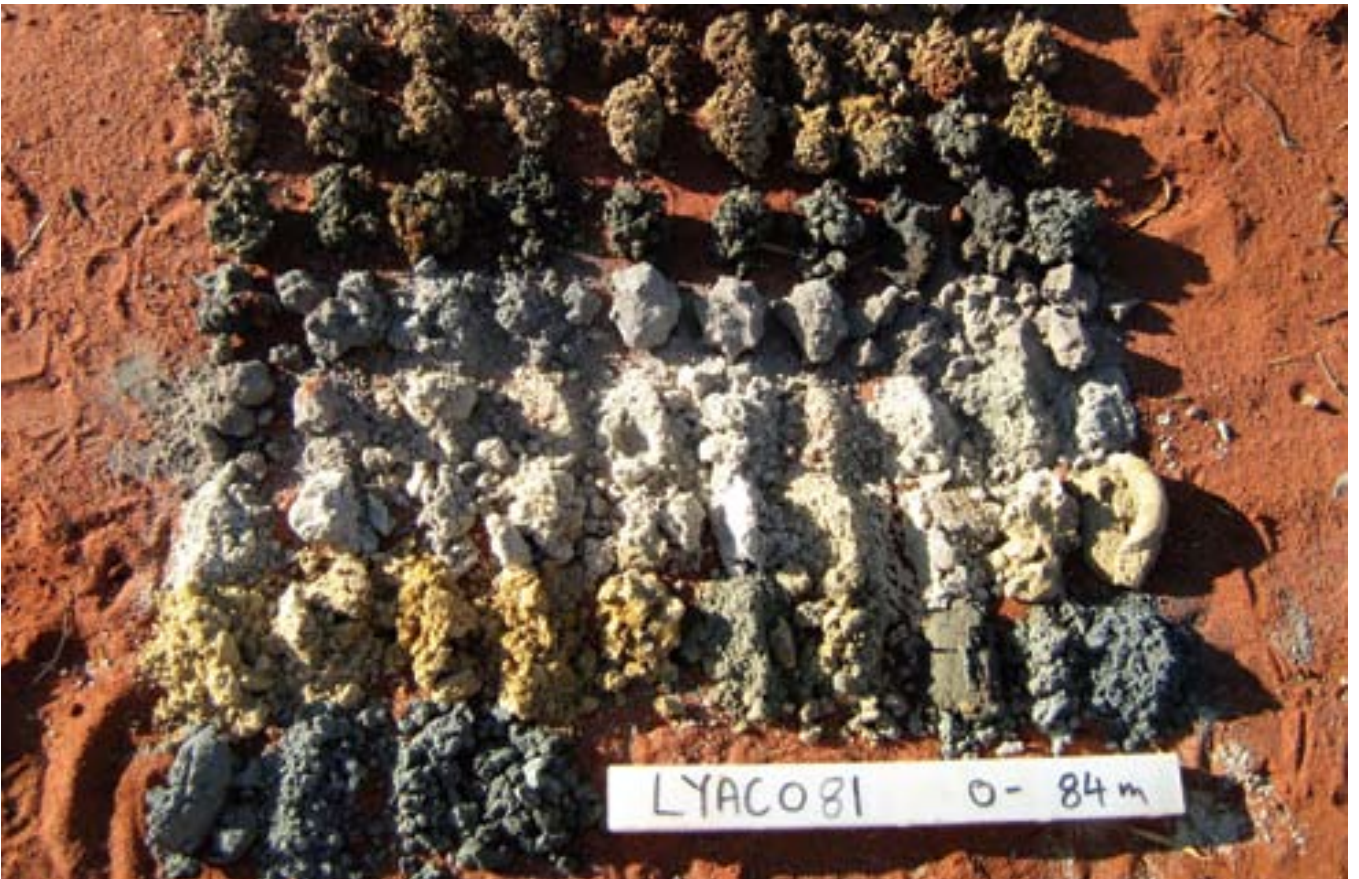
Figure 4. Carley Bore (Nyang Project). Drill spoil pile showing colour changes down through profile due to multiple red-ox zones (LYAC081 7399800N 295100E)
