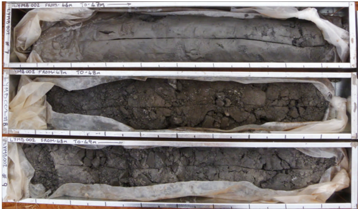
Figure 2 – Sonic core (LYMB002 46-49m) drilled at Carley Bore in July 2011 illustrating near-complete core recovery from semi-consolidated, uranium-mineralised reduced sediments in the ore zone
