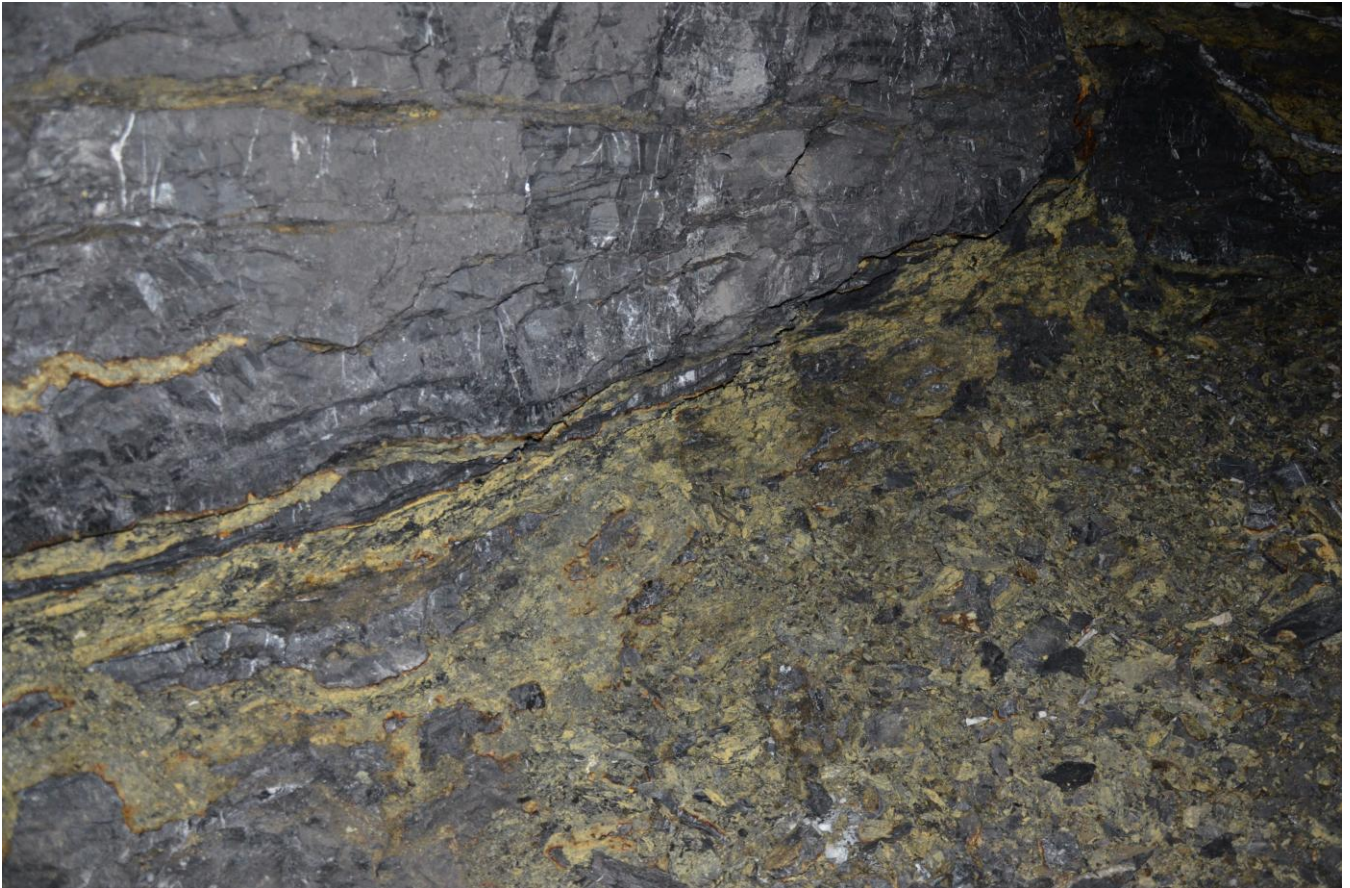
Panel 7: Ore-hanging wall contact 940RL – Grade control intersections in this area have returned grades of up to 14.4m grading 15.3% Zinc and 1.9% Lead (refer 3 June 2014 ASX announcement)
