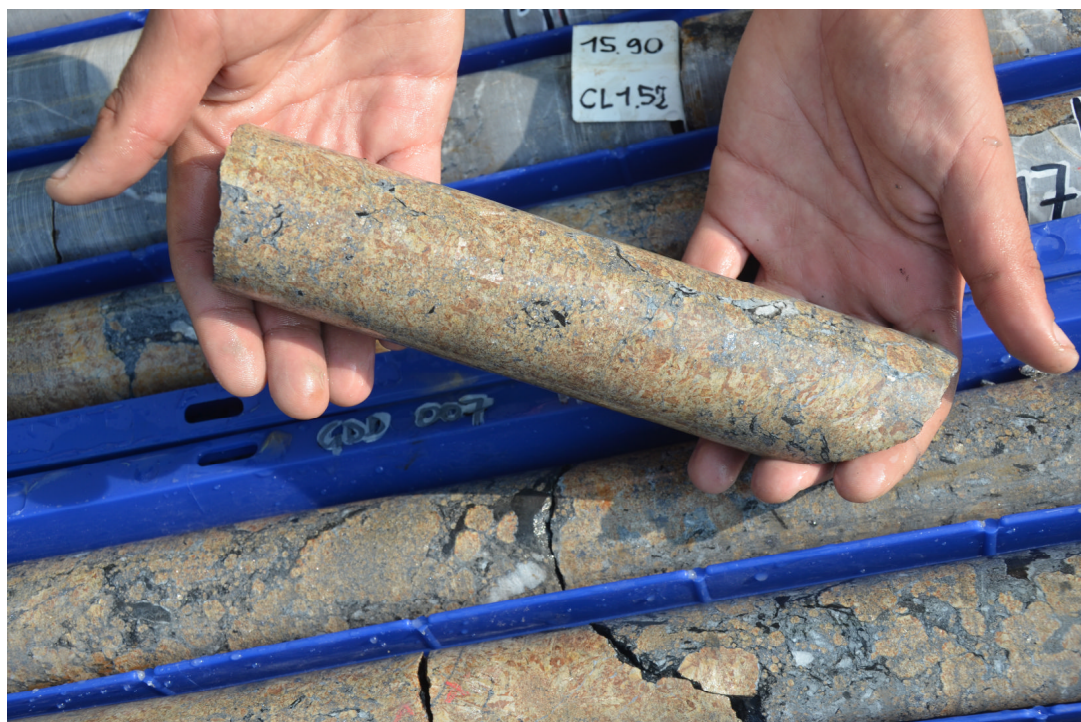
Figure 1: Massive zinc sulphides with sphalerite (brown) and galena (grey) in GDD007
