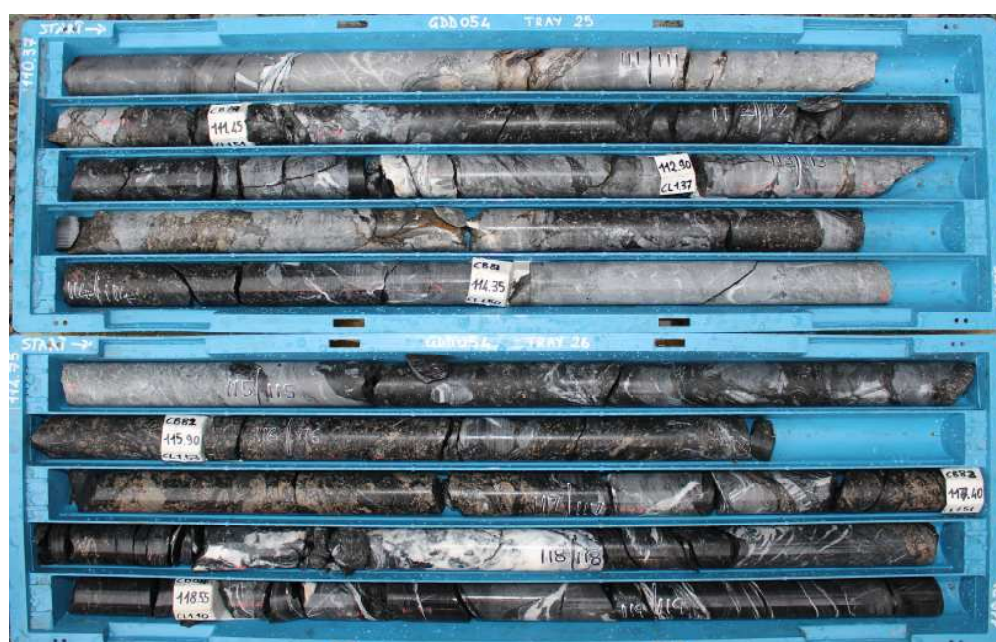
Disseminated to semi-massive zinc sulphides in GDD054
