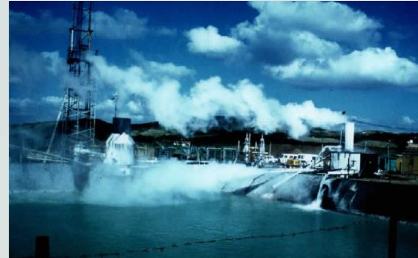
Top: Geothermal pilot plant production test C1 well (1981-82) [Source: STEAM 2023] Bottom: Some of the C1 pipe work showing natural precipitation of minerals (scale) from brine [Source: STEAM June 2023]
