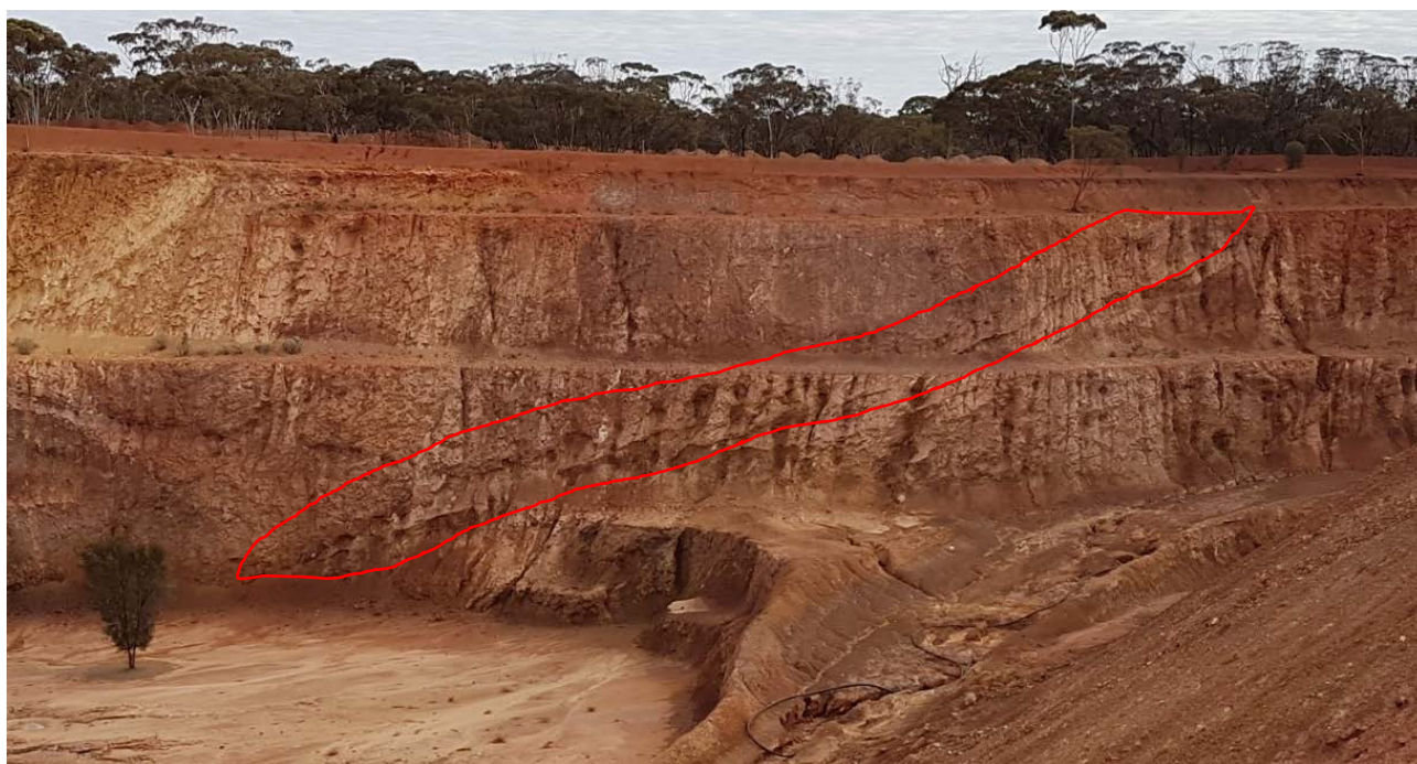
Figure 2: Photo looking at the north west wall of the Fingals Fortune open pit. Low angle veining is highlighted within the pit walls.
