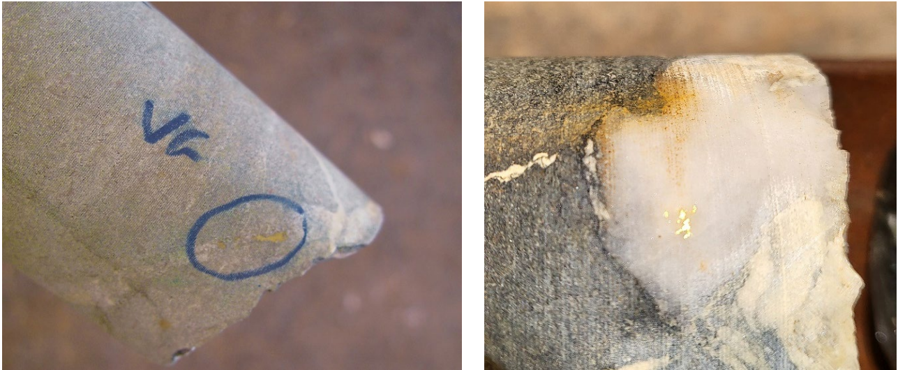
Figure 7: Core photo of 22PGRD019 (left) at ~115m depth and 22PGRD010 (right) at ~49m depth showing visible gold in a quartz vein within the Paulsens Mine Gabbro. Assays for this hole are expected in December 2022.
