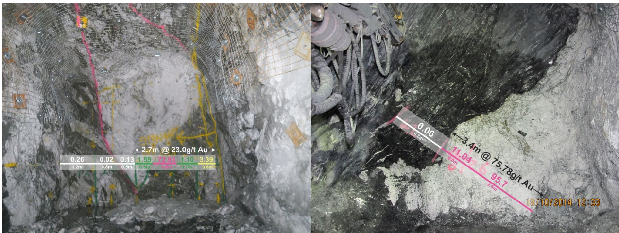
Figure 2: Photo of face 766_400_12 (refer Figure 5) with a composite sample of 2.7m @ 23.00g/t Au (left) and face 441_700_12 (refer Figure 6) with a composite sample of 3.4m @ 75.78g/t Au (right). Neither of these drives were ever stoped with mineralisation not closed off above.
