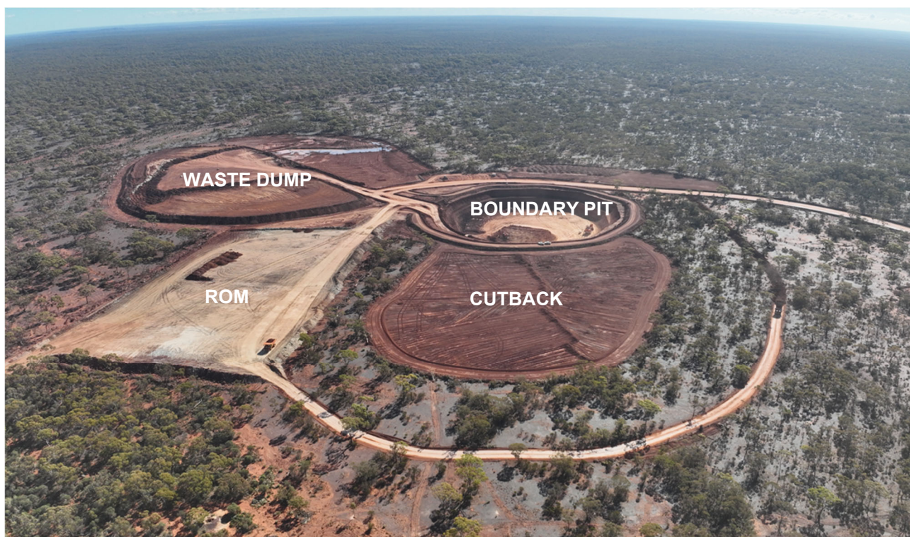
Figure 5: Boundary open pit (looking north) has been mined to 370mRL and topsoil stripping is complete.
