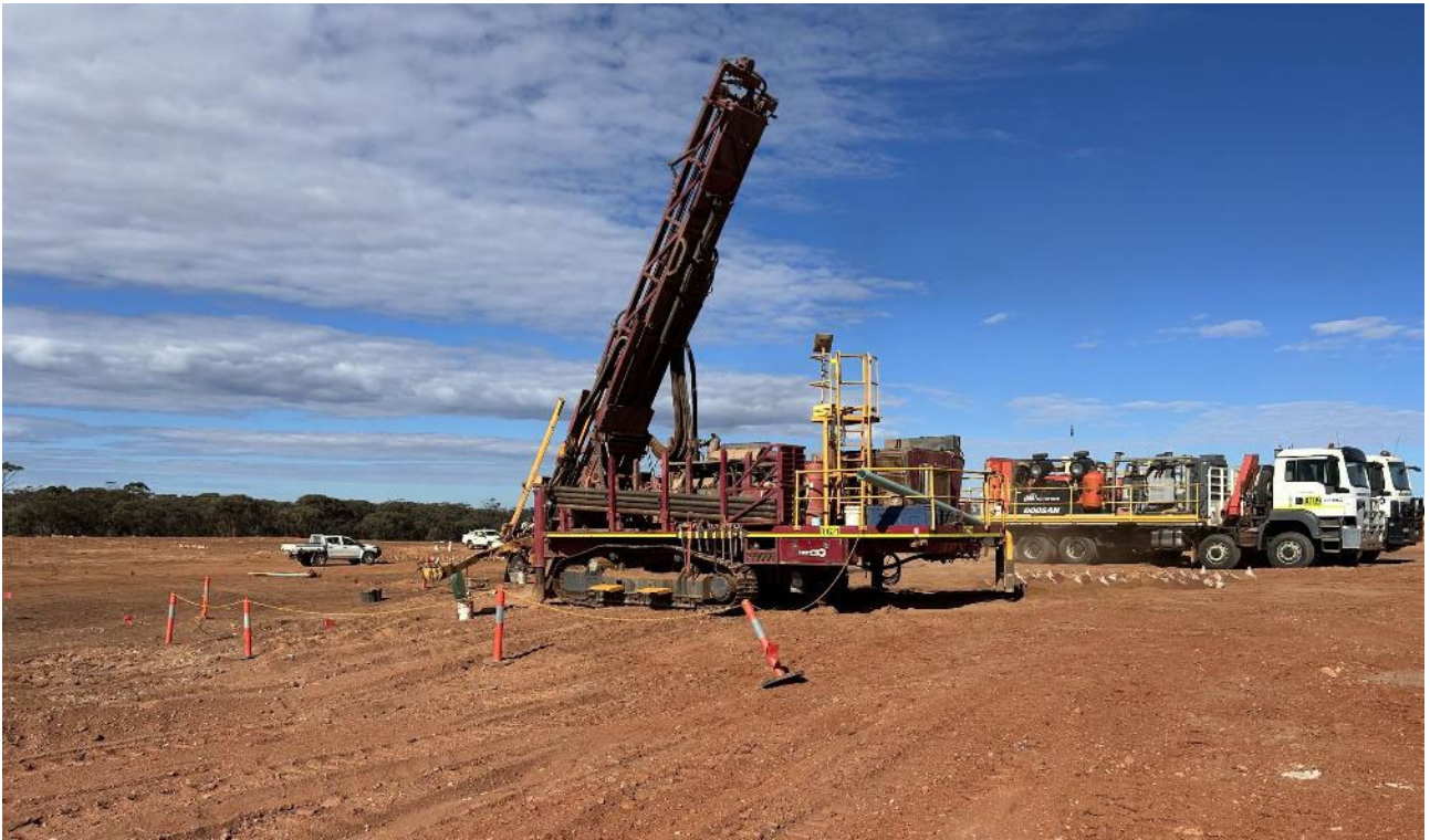
Figure 3: Grade control drilling at Fingals is underway, concurrent with hydrogeological studies for future expansion of the pit.
