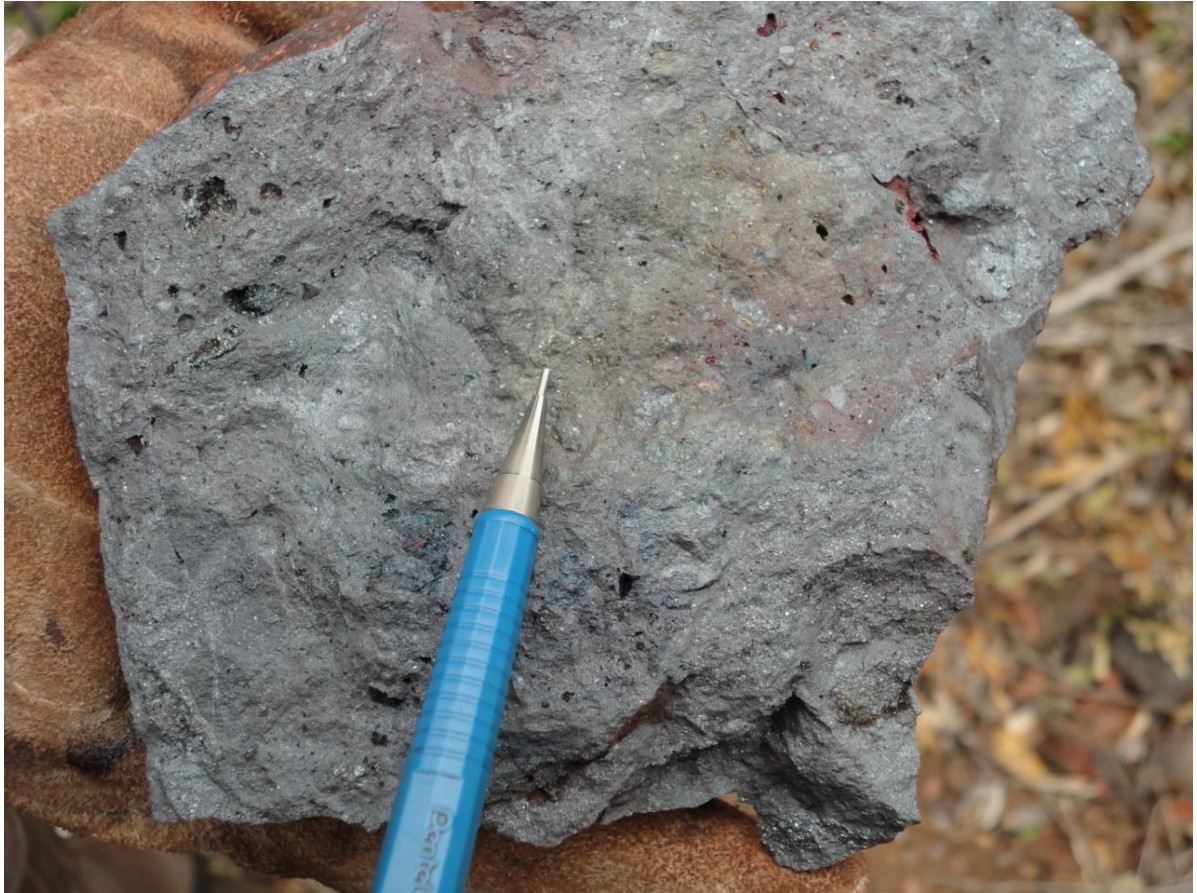
Photo: A close up of a hematite surface sample showing the porous nature of the mineralisation.
