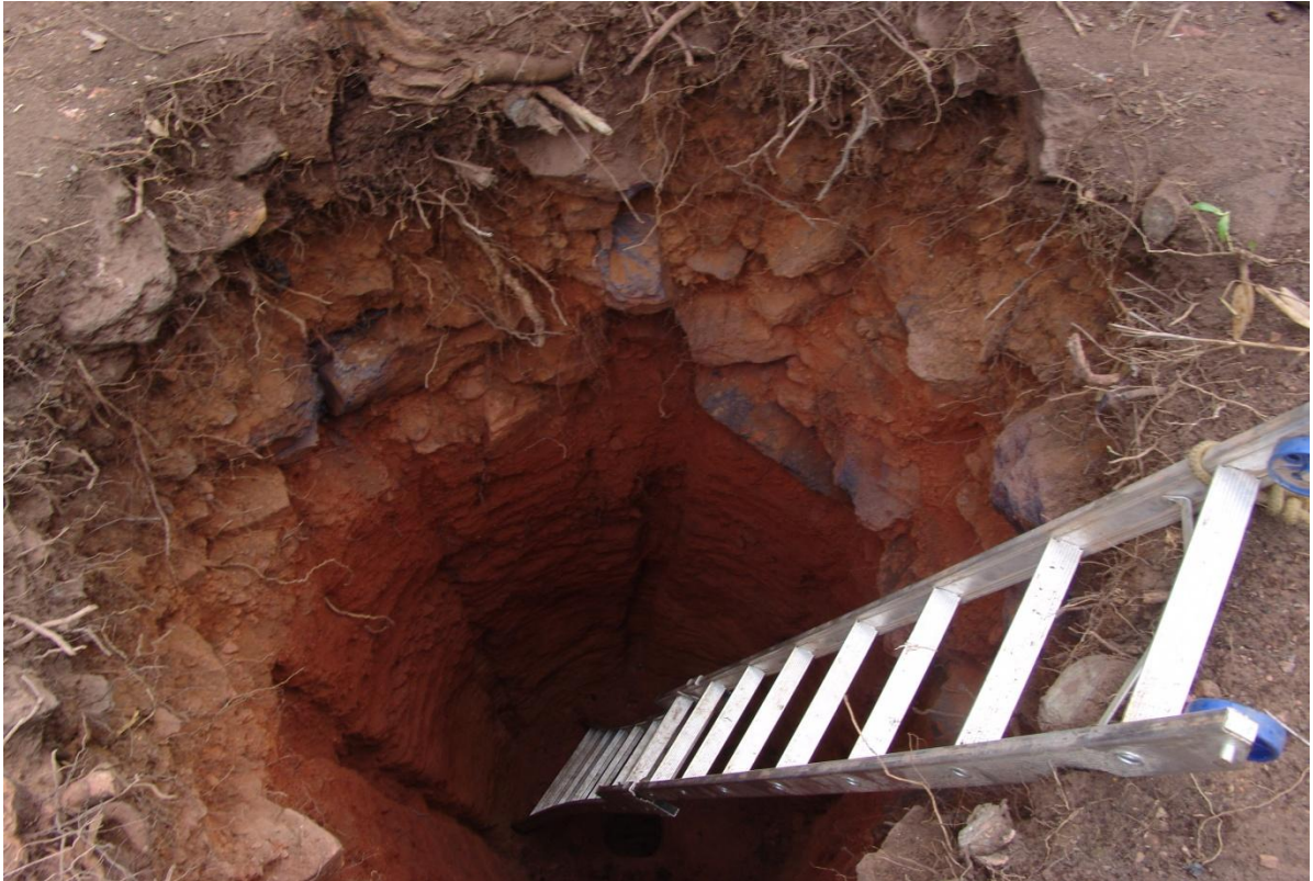
Photo: QXD Pit 2 completed to a depth of 5.25m highlighting where some channel samples have been taken.
