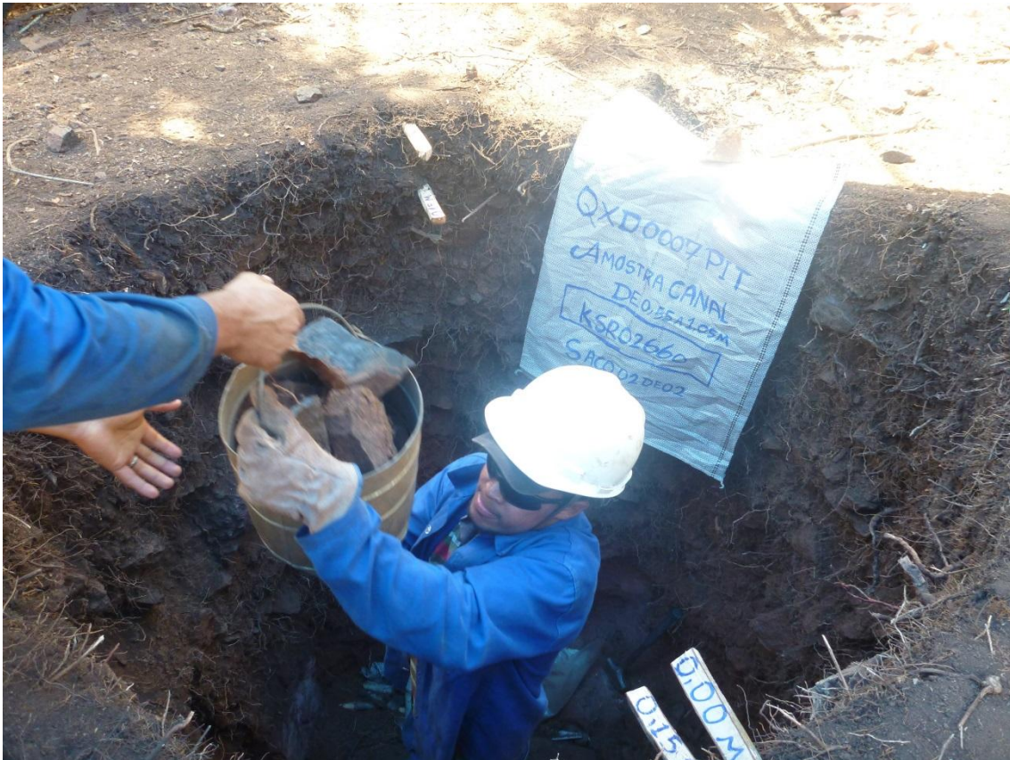
Photo: Channel sample with hematite cobbles being taken from 0.55 to 1.05m in QXD Pit 7.
