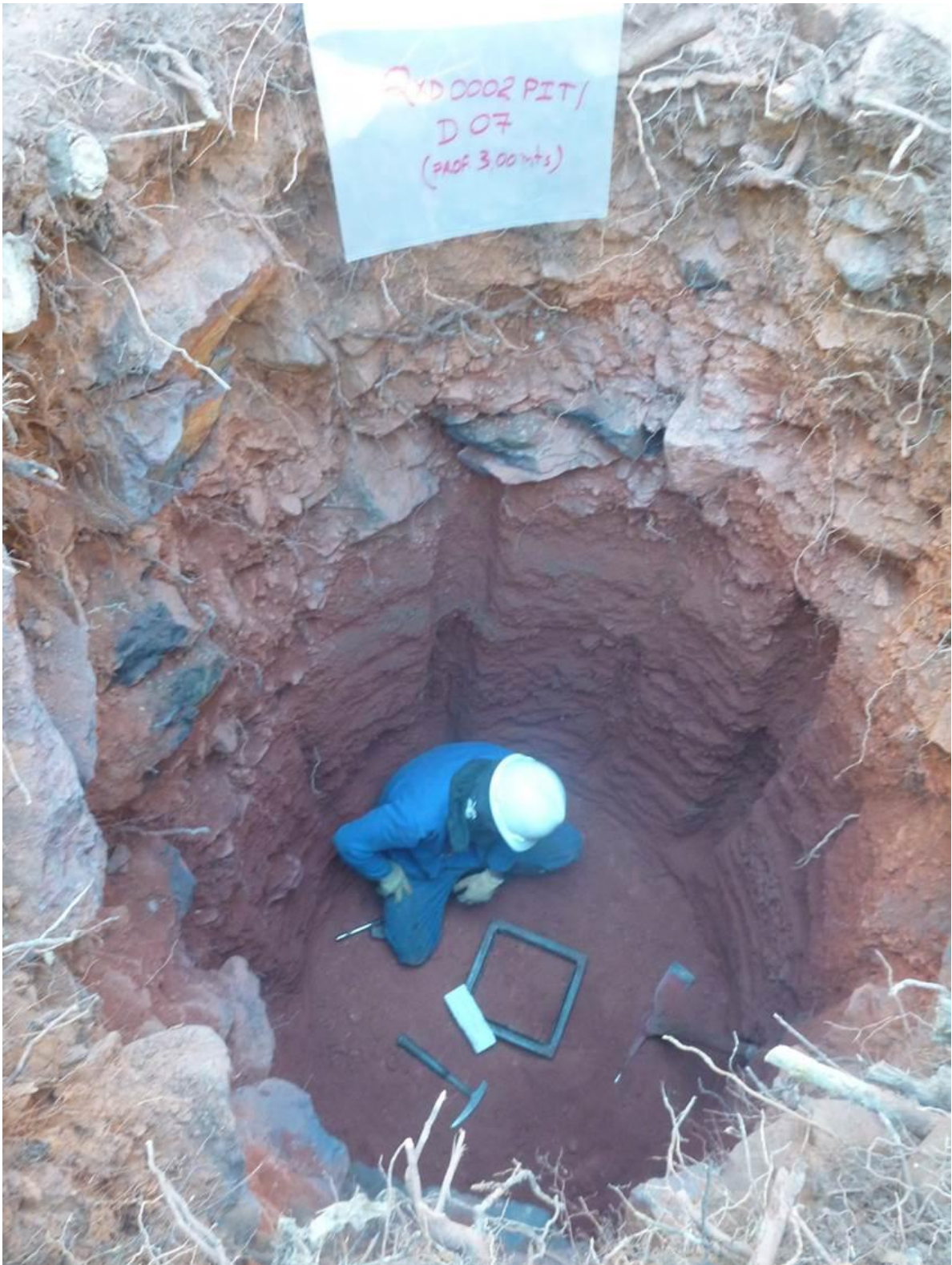
Photo: Sample collecting for density tests at 3.0m deep, in the bottom of QXD Pit 2. Sampled channels are also evidenced at the pit's wall.
