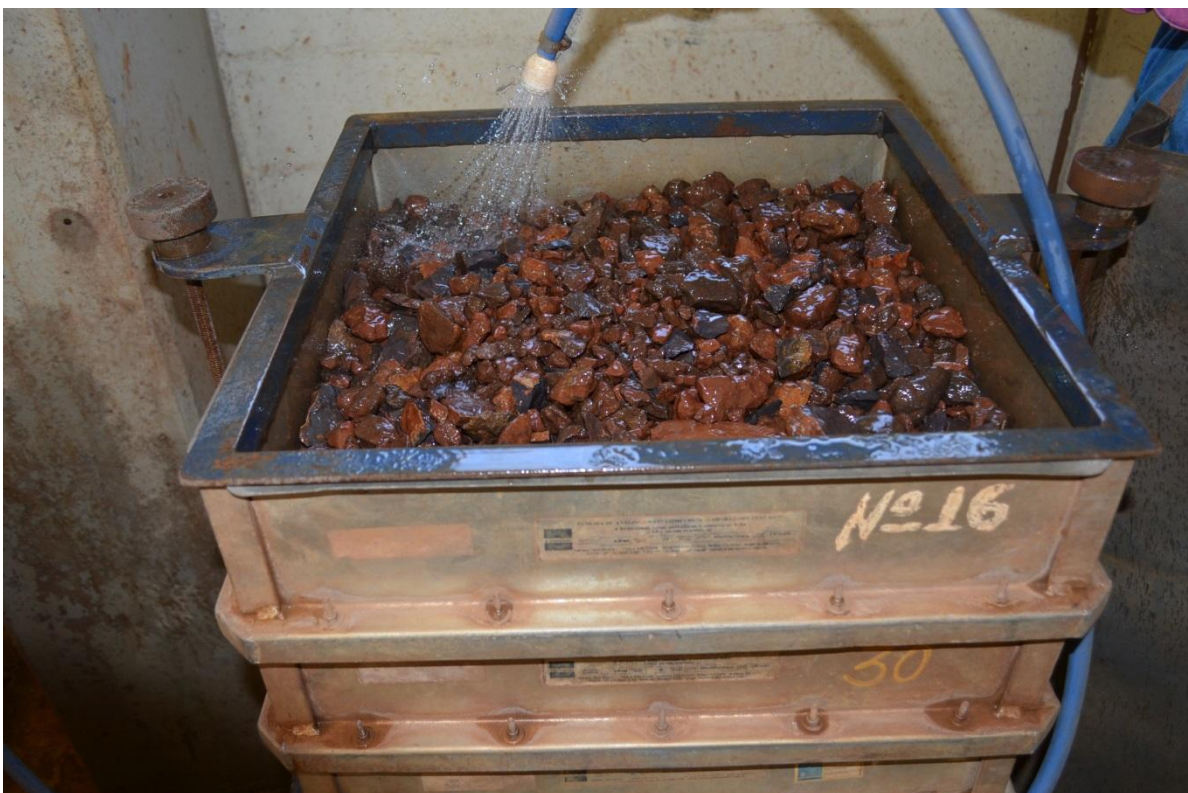
Photo: The 10/12 aliquot wet sieving with four sieves grids sizes set.
