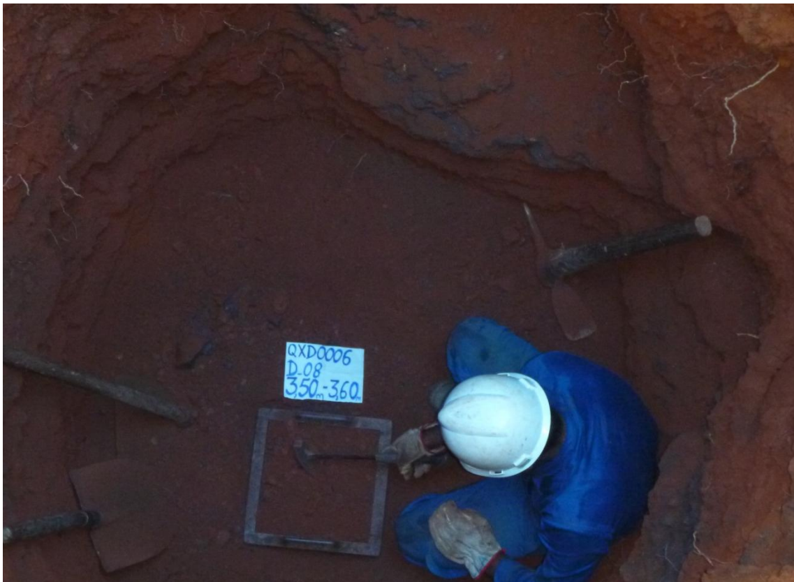
Photo: A sample for density tests being taken from QXD Pit 6.
