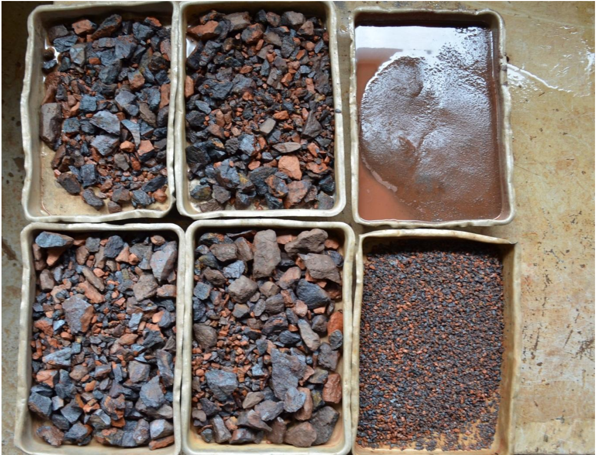
Photo: Part of the size fractionated material obtained by wet sieving over 6.300mm; 1.000mm and 0.149mm.
