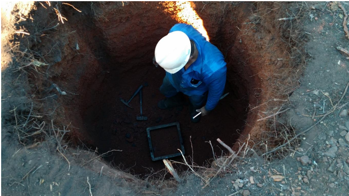
Photo: Taking a 10 litre bulk density sample at 2.0m depth from QXN Pit 1.
