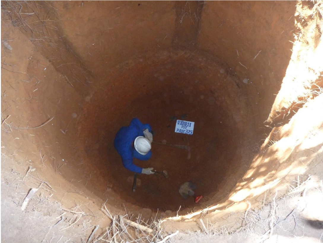
Photo: Digging work progressing within QXD Pit 11 at 3.75m deep.
