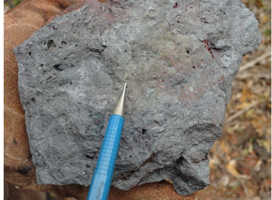
Photo: A surface sample showing the porous nature of the high grade DSO hematite mineralisation.
