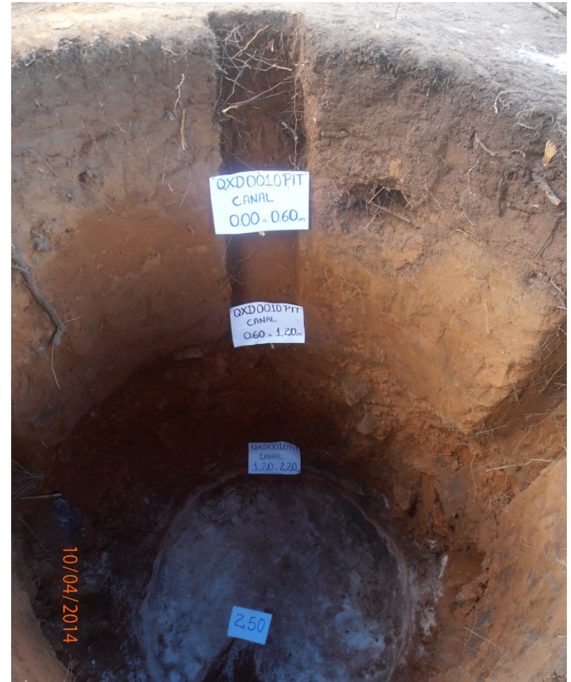
Photo: Channel samples taken from the walls of QXD Pit #10.
