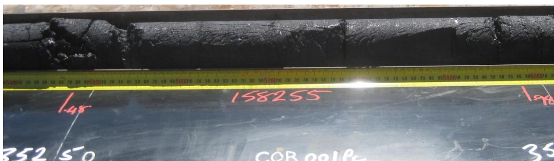
Figure 1. Core from the Mammoth seam in hole COR001PC
