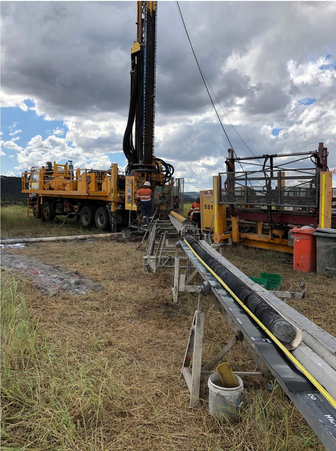
Figure 2. Drill rig with core from HIL049C
