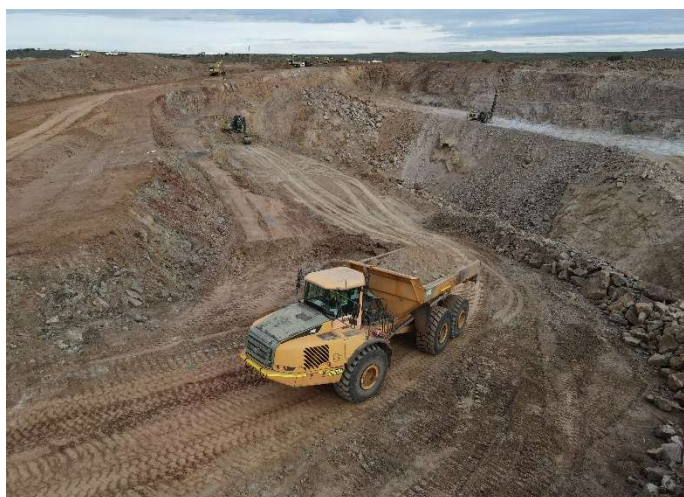
Figures 3 & 4 – Open Pit & ROM operations at the Pinnacles Mine with haul truck loading for transport to Rasp Mill
