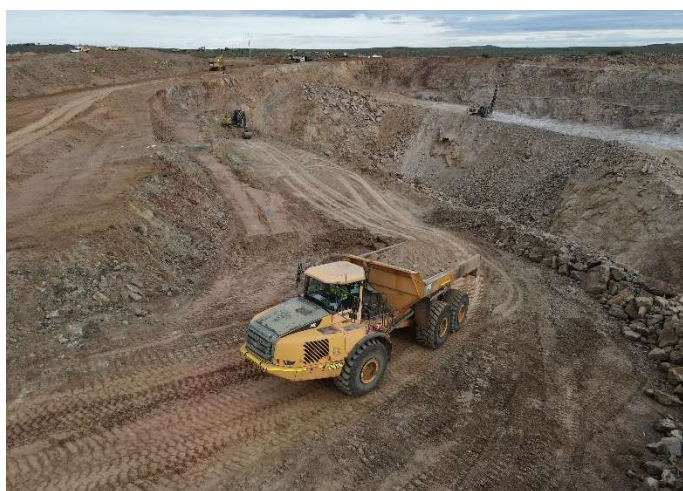
Figures 7 & 8 – Open Pit & ROM operations at the Pinnacles Mine with haul truck loading for transport to Rasp Mill
