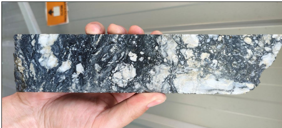
Figure 5. Photo of drill core of hydrothermal breccia with disseminated sulphide and cockade texture that assayed 1m @ 341 g/t Ag, 0.06% Cu, 0.05% Mo within 5m @ 71 g/t Ag, 0.01% Mo from 112.8m (open)
