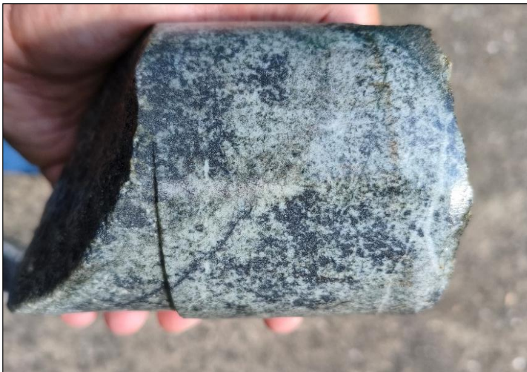
Figure 2. RAV26011 core showing pervasive silicification with bismuthinite-pyrite (dark grey) assaying 1m @ 37.8 g/t Au, 1.7 g/t Ag, 0.6% Bi within 2m @ 21.6 g/t Au, 0.3% Bi from 47m and open in all directions with assays pending below intersection.
