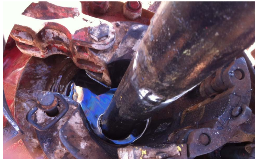
Oil from formation floating in the annulus at the rig floor at Backreef-1
