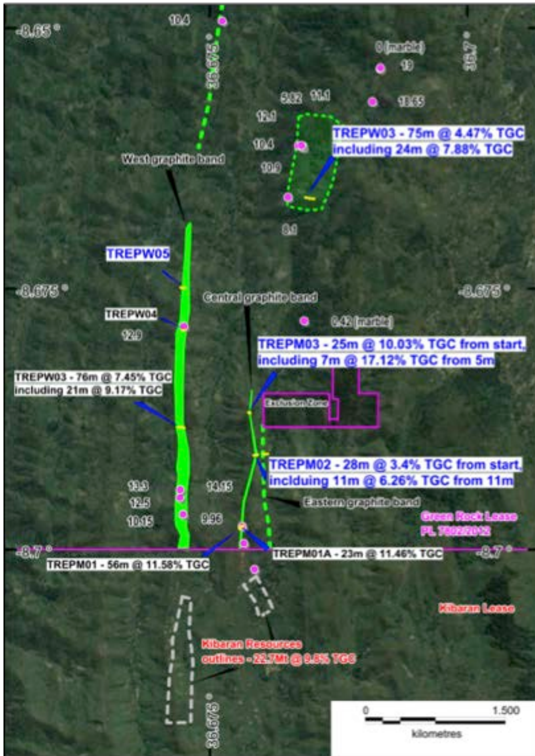
Figure 1. Epanko North trenched area showing trench locations
