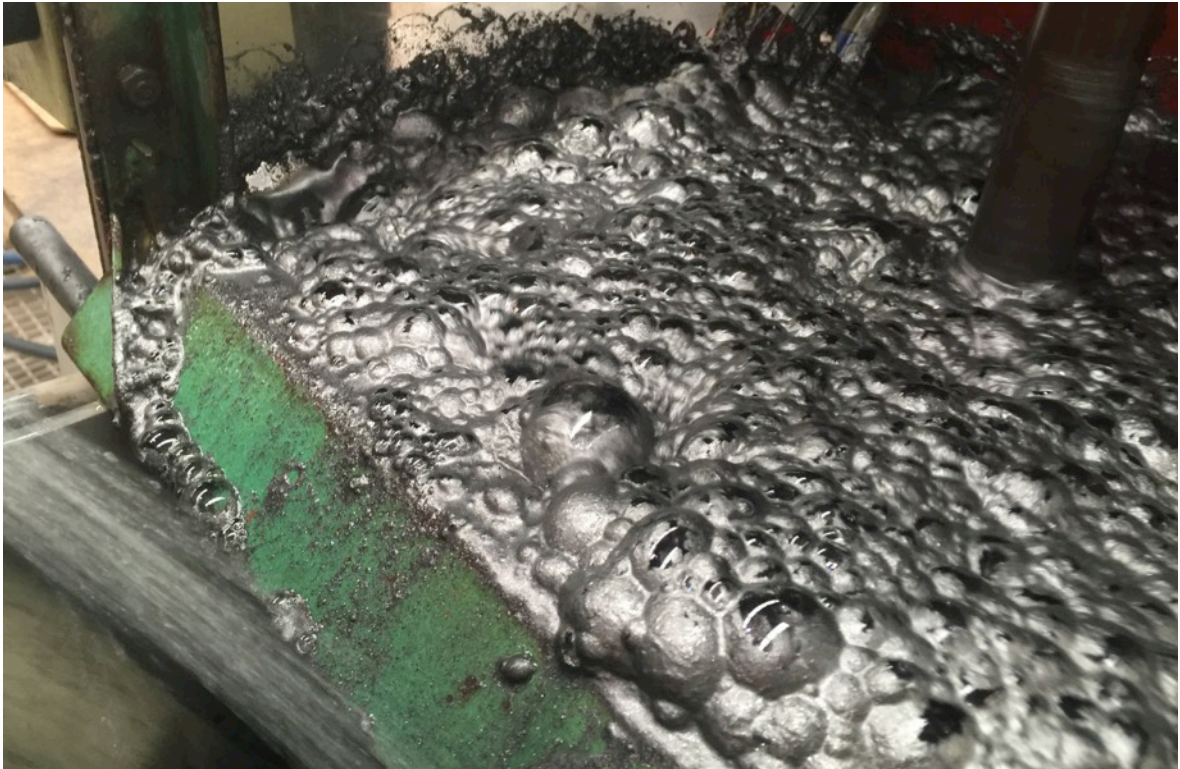
Photos 1&2. Float cell in operation with Ulanzi primary feed (above). Flake graphite concentrate ready for sizing analysis (below).
