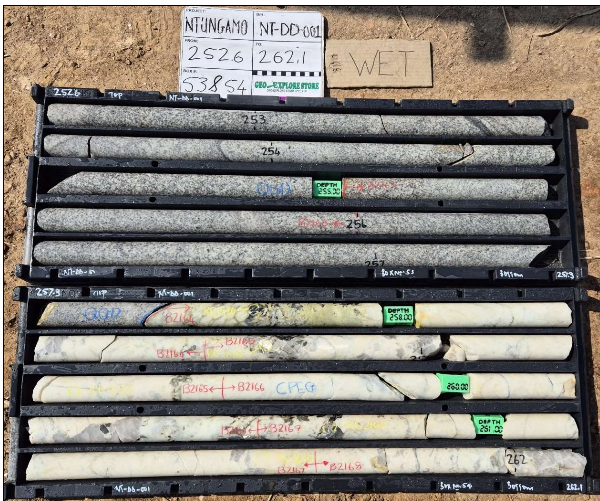
Figure 1: Photo of marked-up core from hole NT-DD-001 from 252.6m to 262.1m. Note the finer-grained, grey coloured quartz granitoid (QGD) on top, in contrast to the mostly white coloured, coarse-grained pegmatite (CPEG) at the bottom of the photo. XRF readings show an increase in anomalous rubidium values in the CPEG (mostly within the mica and feldspar minerals). Spot readings from the XRF are marked in yellow on the core where relevant.
