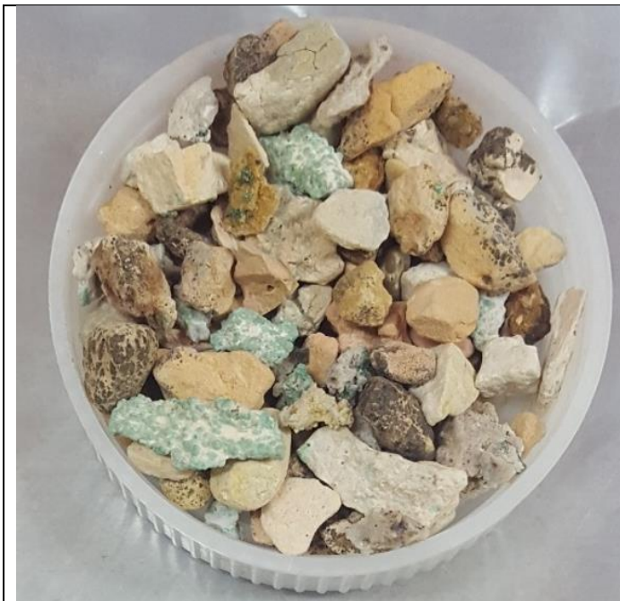
Figure 5: > 3.35mm fraction from testwork on core – large fragments with malachite (green)
