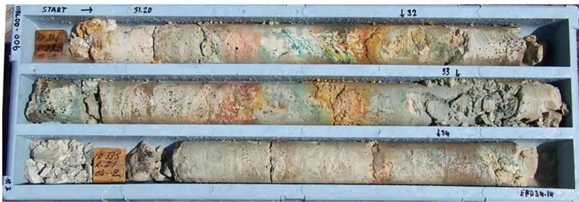
Figure 4: Blebs and disseminated malachite in Sandfire diamond hole 11BLDD006
