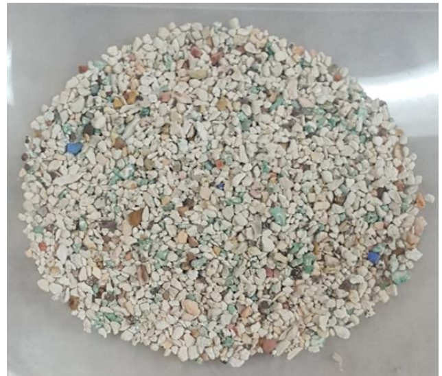
Figure 6: > 0.85mm size fraction from testwork on core – visible rounded pieces of malachite (green) and azurite (blue)
