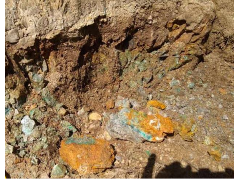
Figure 3: Verification channel sampling at Coaxtlahuacan, over copper-gold mineralised zone. Observed malachite and chalcocite
