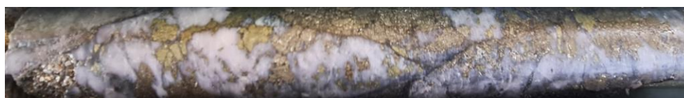
Figure 1 – Drill core from drill Hole DTDD009 showing quartz-chalcopyrite vein material grading 171.8 g/t Au, 56.4 g/t Ag & 5.28% Cu
