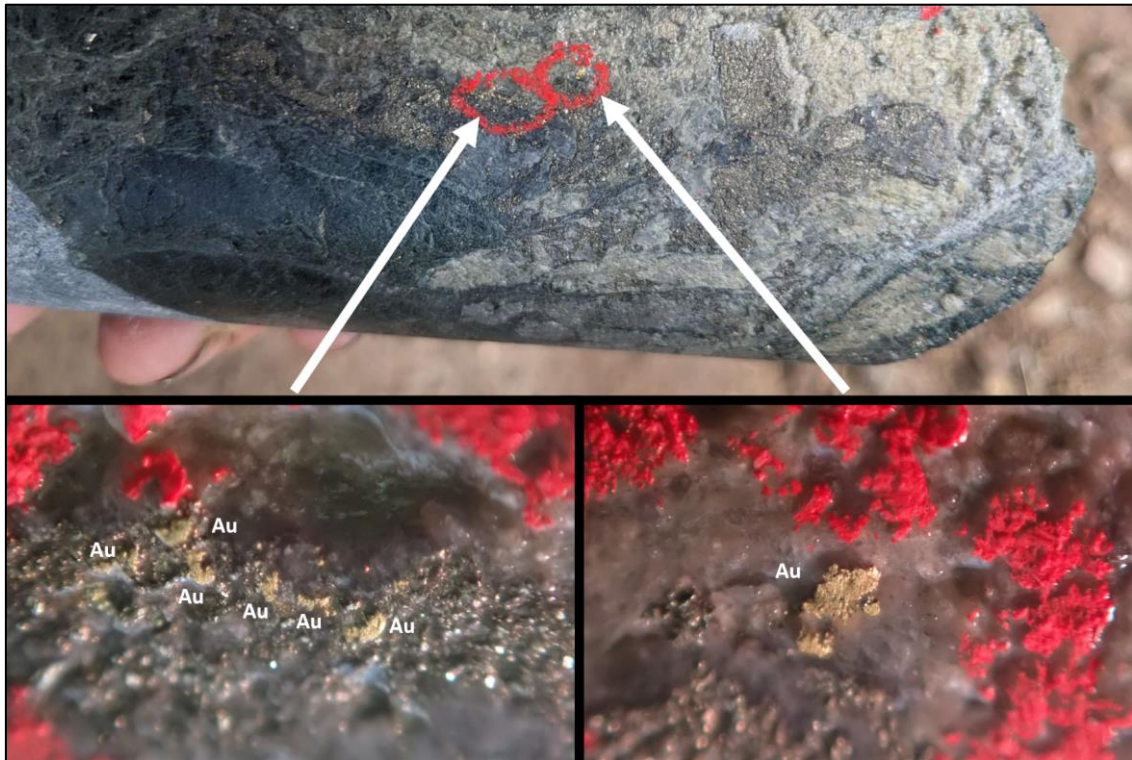
Figure 3 – Pyritic shear zone intersected in DTDD023A with visible gold (158.0 – 158.2m).
