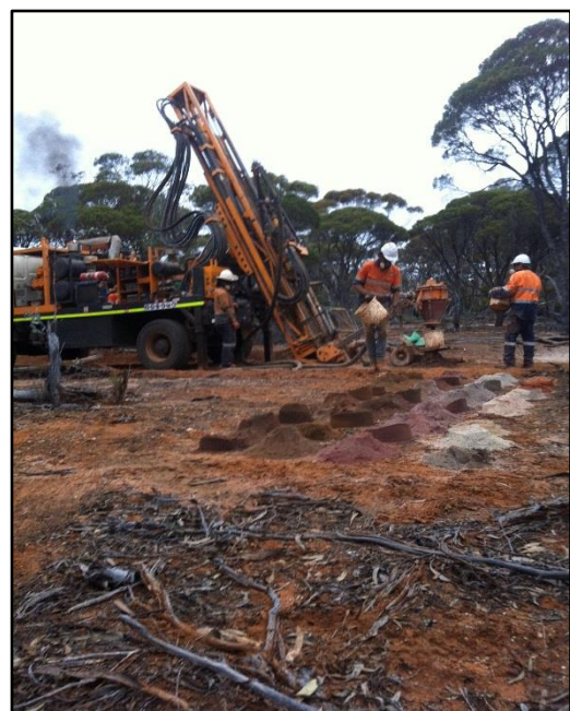
Aircore Drilling at Symons Hill – Oct 2016
