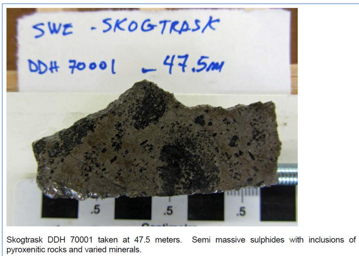
Figure 5. Portion of the core sampled from DDH 7001 over the interval 46.3 to 48.3m. The interval assayed 1.1% Nickel and 0.2 % Cu.
