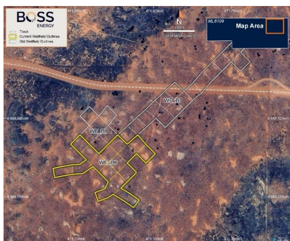
Figure 3: East Kalkaroo showing previous wellfield design (left) and the current trial wellfield design (right). Note: Each 'square' outline in the above figures represents a 'pattern' which consists of four injection wells on each corner of the square and an extraction in the centre (five-spot pattern). The previous pattern size B6, B7 and B9 was 42m x 42m (30m injection to extraction well). The current trial design of EKT1 has a pattern size of 85m x 85m (60m injection to extraction well).
