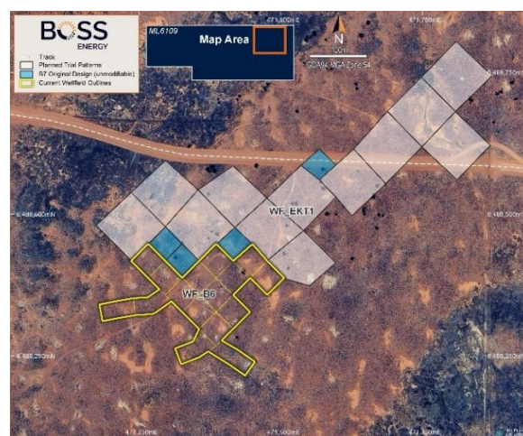
Figure 3: East Kalkaroo showing previous wellfield design (left) and the current trial wellfield design (right). Note: Each 'square' outline in the above figures represents a 'pattern' which consists of four injection wells on each corner of the square and an extraction in the centre (five-spot pattern). The previous pattern size B6, B7 and B9 was 42m x 42m (30m injection to extraction well). The current trial design of EKT1 has a pattern size of 85m x 85m (60m injection to extraction well).
