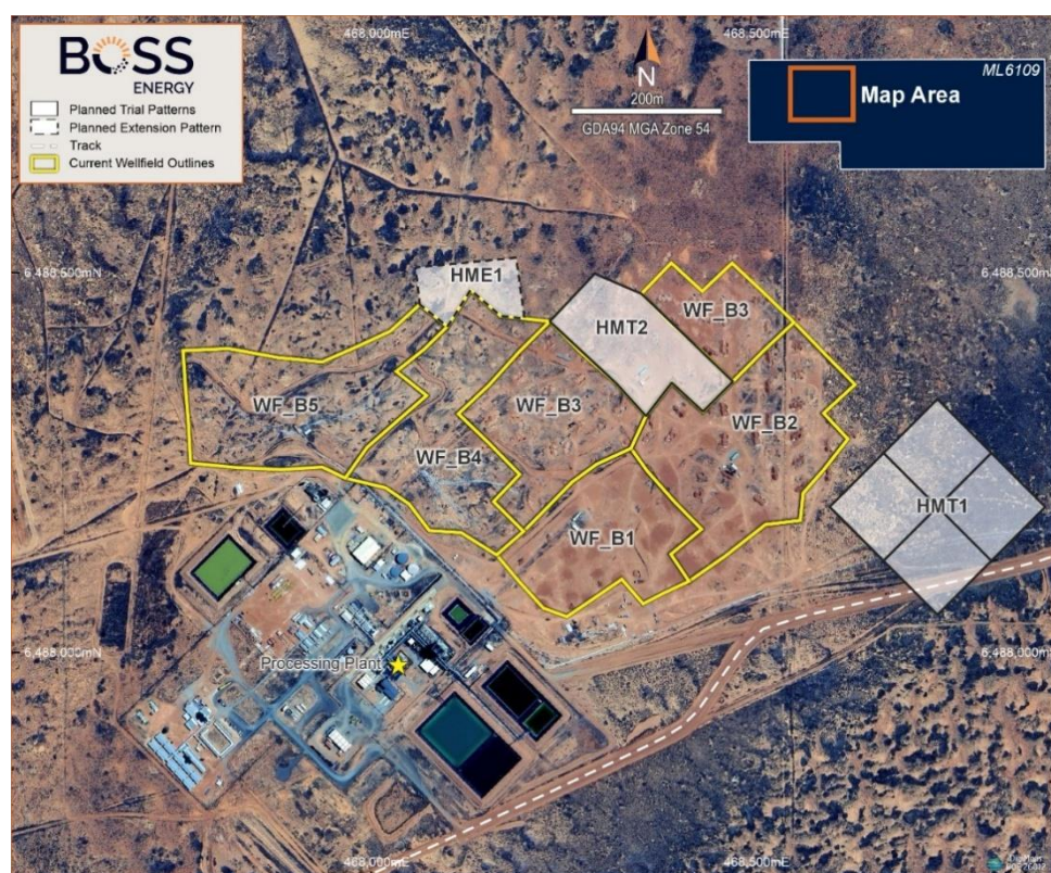
Figure 4: Wellfield design on the Honeymoon Domain showing both the trial (HMT1 & HMT2) and extension patterns (HME1). The current wellfield design of B1-B5 has a pattern size of 56m x 56m (40m injection to extraction well), the trial design of HMT1 has a pattern size of 100m x 100m (71m injection to extraction well) and HMT2 has a pattern size of 90m x 90m (55m from injection to extraction well), albeit an irregular shape. HME1 consists of two additional extraction wells, which are 40m away from the existing injection wells.
