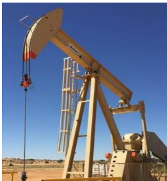
Variable speed beam pump installation in ex PEL 91 1. Year-to-date for nine month periods to 31 March
