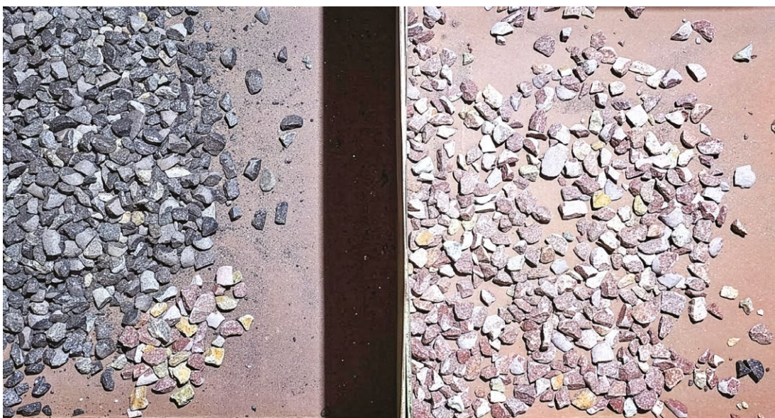
Drop (left) and Eject (right) sorter fragments showing clear separation of dark ultra high-grade Monte Alto mineralisation.
