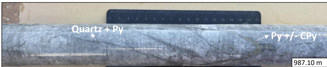
Figure 5: Core photos from Tambo South drill hole TMT-TSU-DD-001 showing quartz veins with pyrite (Py 0.8%) +/- chalcopyrite (Cpy 0.01%; visual abundances estimated as volume-percent from 987m to 989m).
