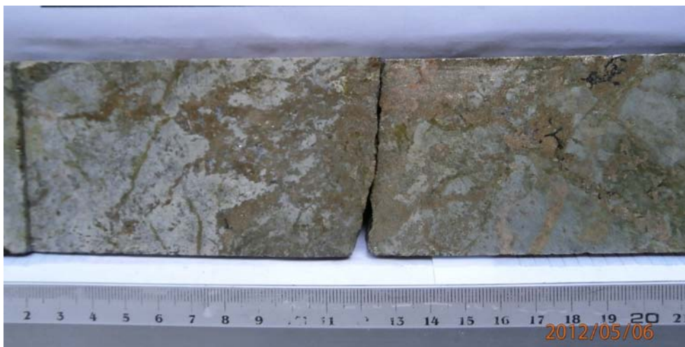
Figure 2 - BCPDH00001 69.30m garnet- pyrrhotite skarn mineralisation. 69.00m-69.70m @ 0.86% Cu
