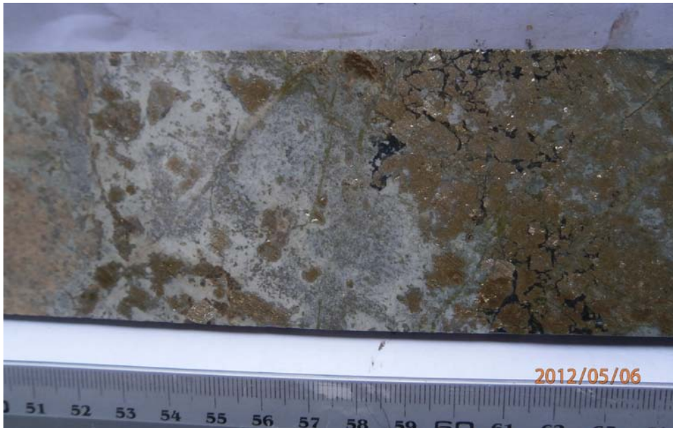
Figure 1 - BCPDH00001 66.50m garnet - pyrrhotite skarn mineralisation. 66.40 m - 67.40m @ 3.89% Cu
