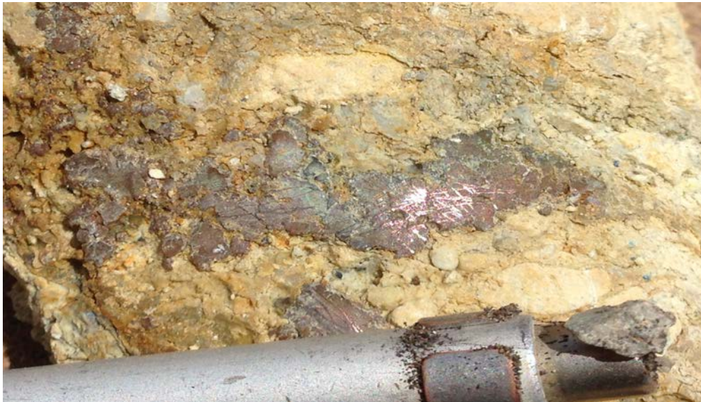
Figure 2 – Native copper in drill core from hole RCPDH00012 at 89.55m downhole, beneath the Panga underground mine. Field of view 5cm.
