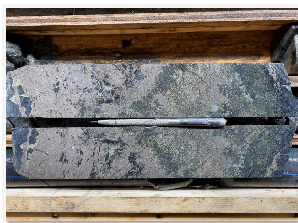
Figure 1 - Core from drill hole JWD21-01 showing Cu-Ni-Co sulfarsenide mineralisation
