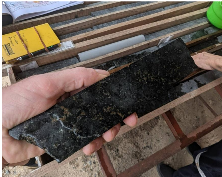
Figure 1.5_2 Disseminated Ni Sulphide Mineralisation in Ban Phuc drilling (Source Sahara 2025)
