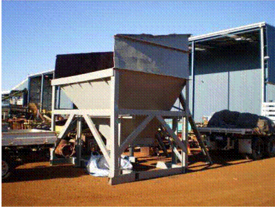
Mill Feed Bin after Surface Treatment
