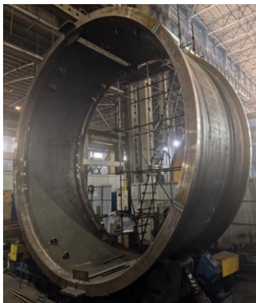
Figure 4 - Steel fabrication underway: SAG mill shell (left) and trunnion (right)
