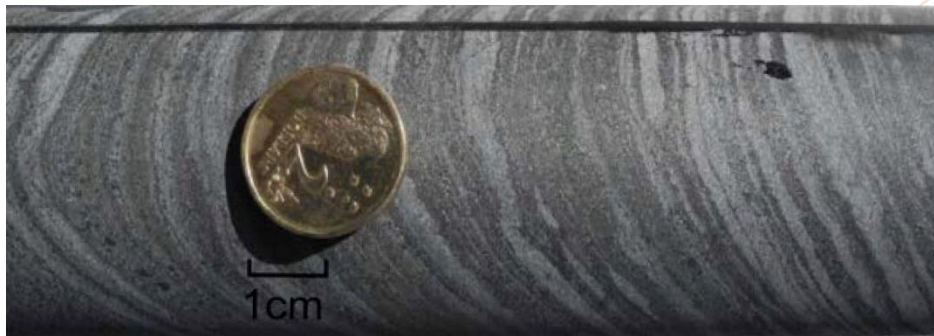
BIF magnetite mineralisation in drill core from hole YS12DD017
