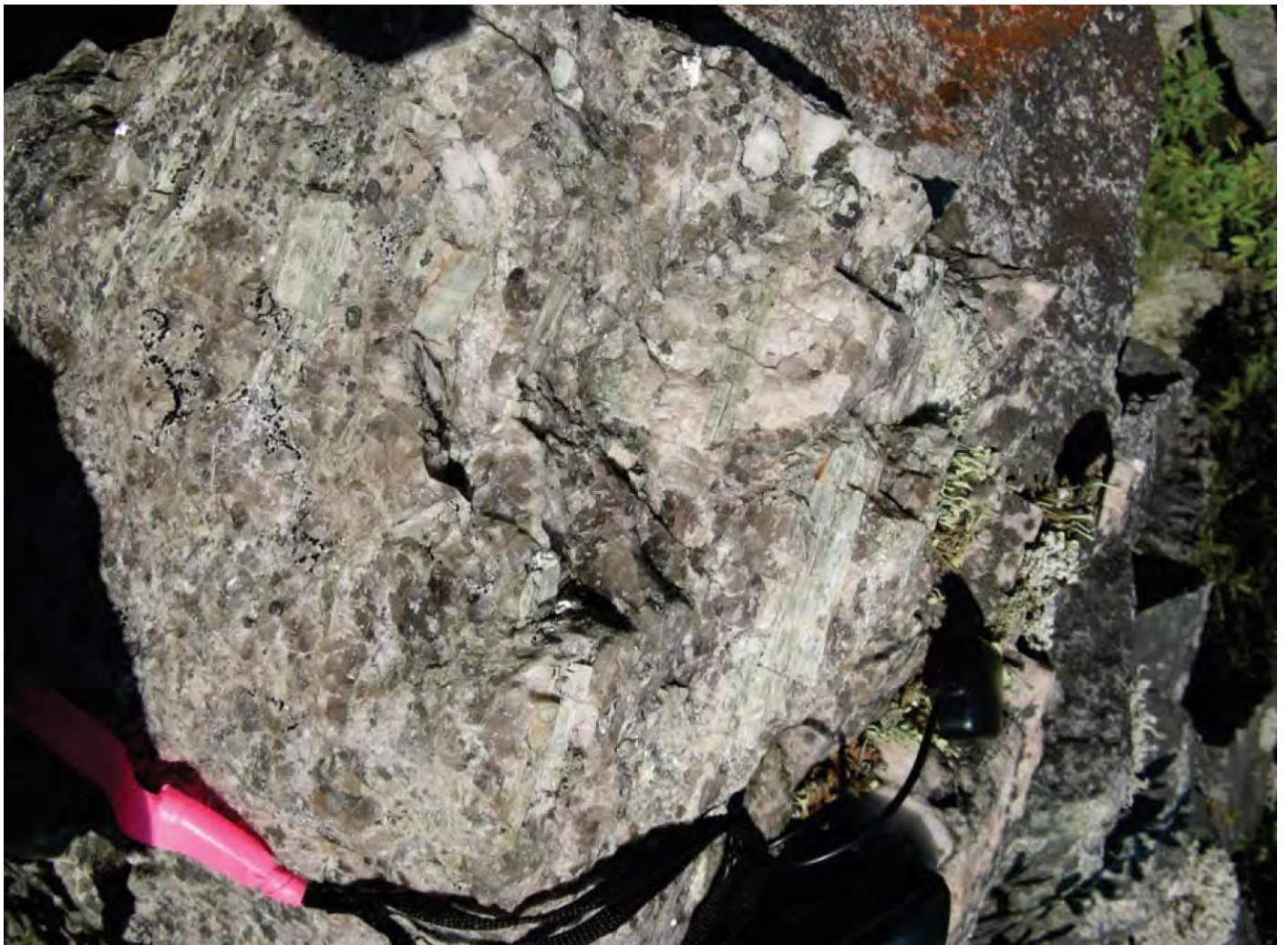
Figure 7: Typical assemblage of spodumene-quartz-feldspar-muscovite observed in granitic pegmatite at the Chubb Project
