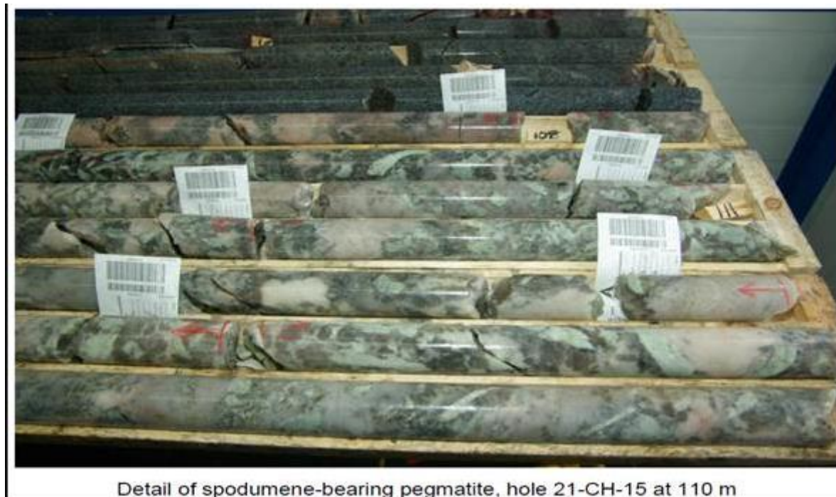
Figure 8: Core Samples from Main Dyke -showing large crystal structure of the spodumene-bearing pegmatites
