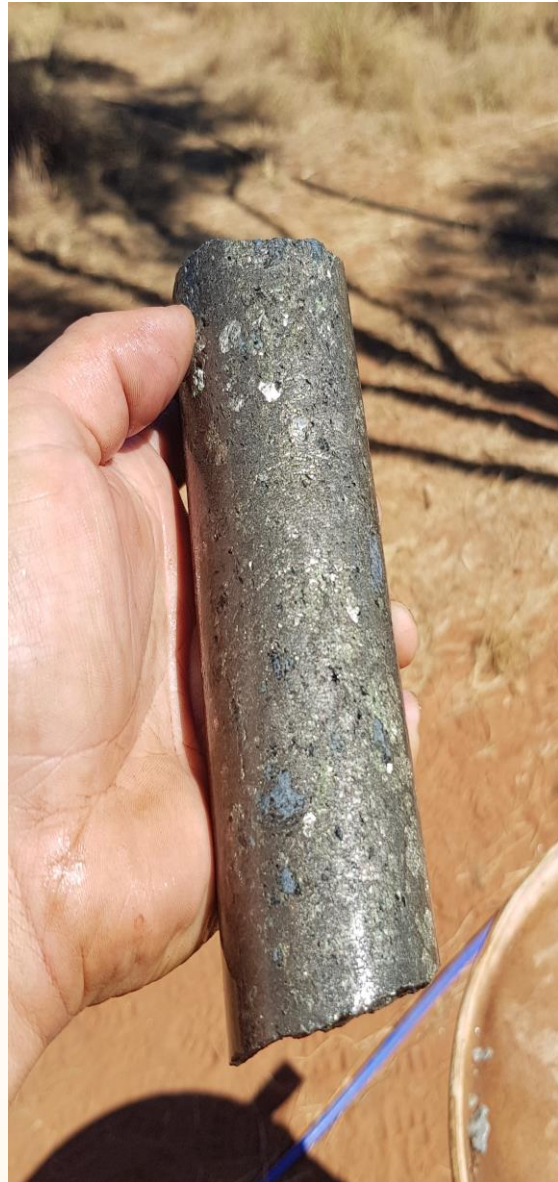
Figure 3. Brecciated massive sulphide from DMDD0018 with visible Pentlandite, Chalcopyrite & Pyrrhotite, photograph is of NQ whole core 237.7-237.85m downhole.
