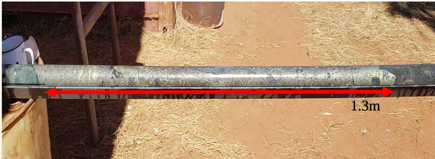
Figure 1. Brecciated massive sulphide interval from DMDD0018, core is NQ, from 236.6-237.9m downhole
