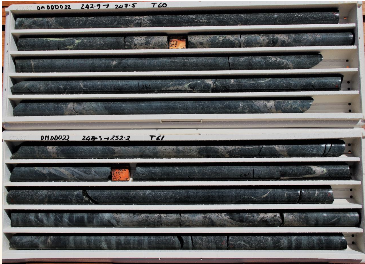
Figure 2. Well-developed 10 metre mineralised interval displaying strong disseminated and moderate net textures and lessor massive sulphide mineralisation from DMDD0022, core is NQ, from 242.9-252.2m downhole.
