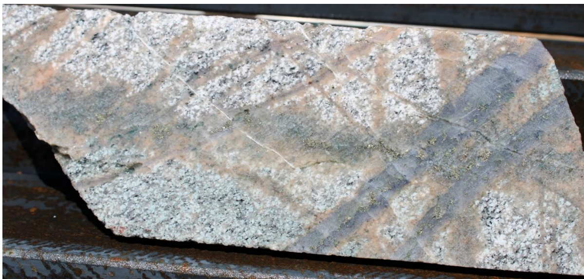
Figure 1: CW0001DD core showing mineralising quartz-pyrite-chalcopyrite-molybdenite+/-bornite sulphide vein stockwork within strongly altered gneissic rock at 546.6m. Pervasive alteration consists of sericite-chlorite-k-feldspar-silica which is also displayed as vein selvages around the sulphides. HQ core is 63.5mm width.
