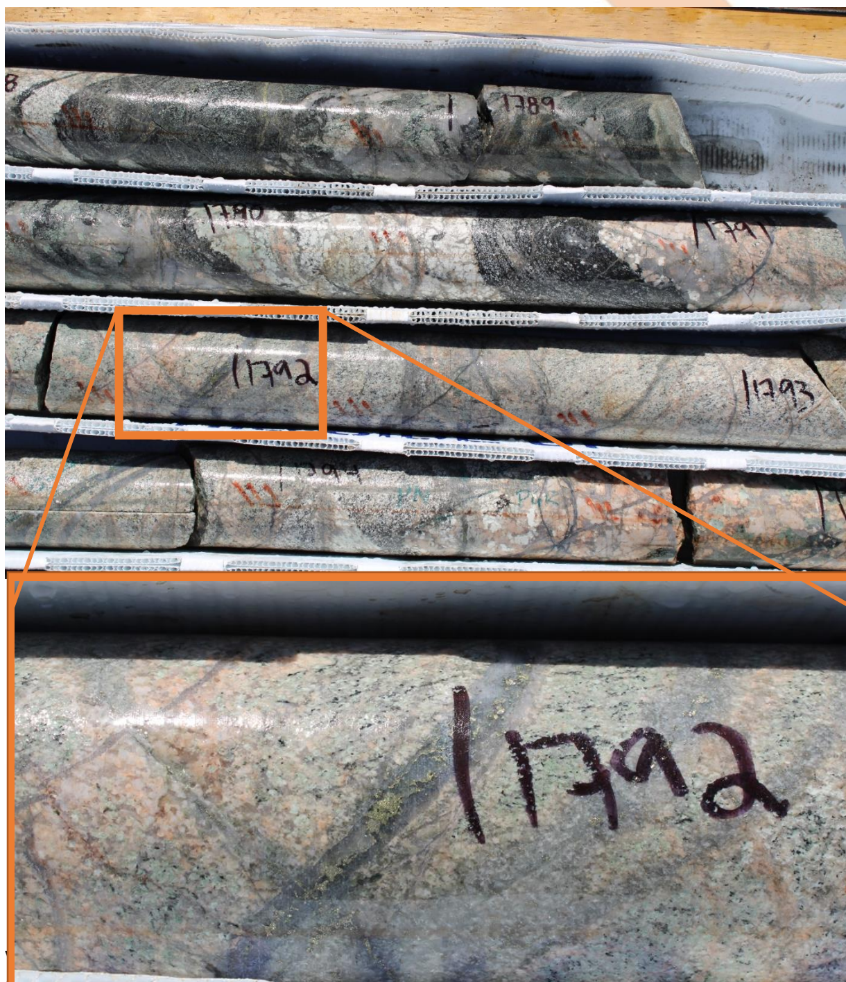
Figure 4 Stockwork quartz-sulphide veins around 546m, including chalcopyrite-pyrite mineralisation within veins and as disseminations. Depth marked in feet (1 metre = 3.281 feet)
