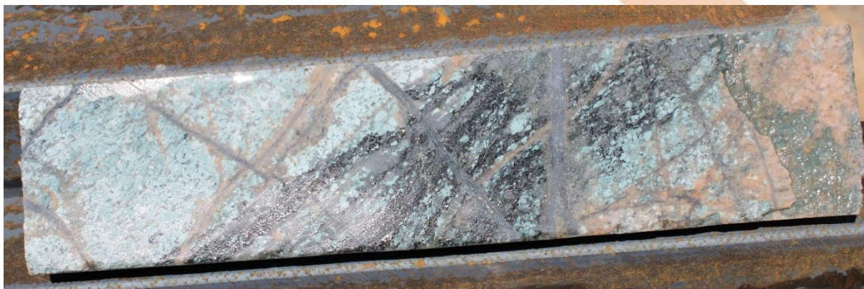
Figure 2: Multi-stage quartz veining with sulphides including pyrite, molybdenite, chalcopyrite and bornite hosted in potassium feldspar-chlorite-sericite-silica altered schist at 562.3m.
