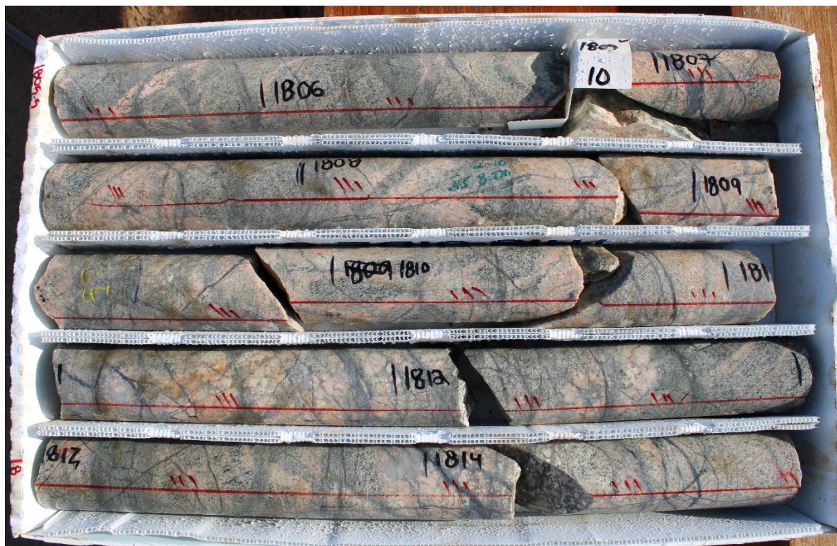
Figure 6: Altered albite-sericite-chlorite-garnet gneissic geology cut and mineralised by multiple phases of intense quartz-sulphide veins, 550 to 554m. Core depth in feet (1 metre = 3.281 feet)
