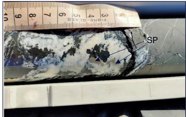
Photos 1 & 2: Examples of field observations of coarse sphalerite (Sp- honey coloured mineral) remobilised in quartz-carbonate veins in diamond holes BRD0006 and BRD0007 drilled in northwestern extensions*
