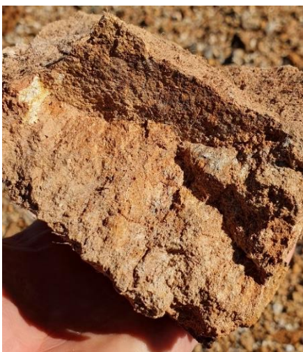
Figure 8 – (left) Field photograph of weathered carbonatite rock chip sample BY23K0360 assaying 1.09 % TREYO (22% NdPr) (right) Field photograph of weathered iron oxide rich pyroxenite or possible ferrocarbonatite rock chip sample LRBY21 with assays returning 263 ppm Sc 2 O 3 and 0.7% TREYO (30% NdPr).
