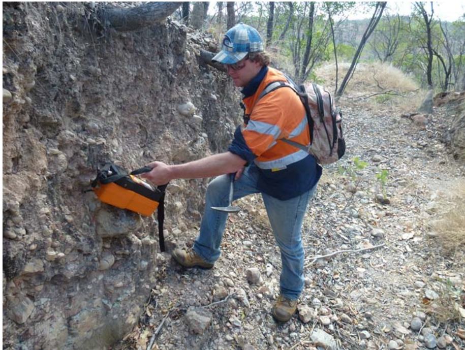
Uranium detection using a differential spectrometer
